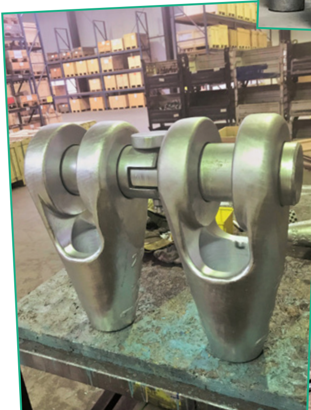
George Washington Bridge Socket (GWBS)
